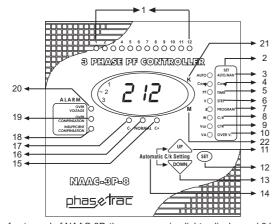
On the front panel of NAAC-3P, there are warning lights, display and 3 buttons for settings.
